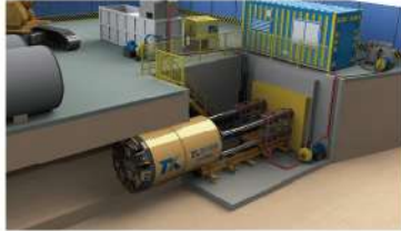
主顶油缸推动顶管机顶进 Jacking in pipe jacking machine
