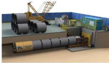
长距离顶进，安放中继间 Install inter jack station
