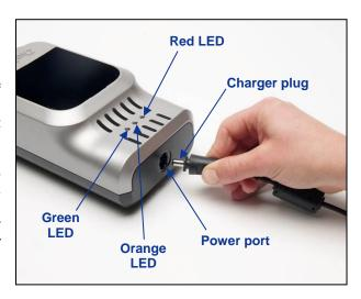
Inserting Charger Plug into Power Port
